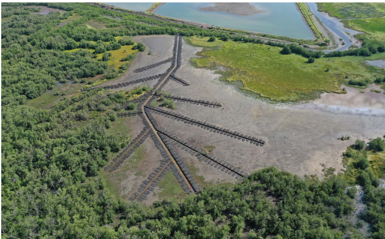
Aerial view of the hydrological restoration taking place on an Operation Wallacea. A main channel has been excavated to feed water across the whole site. Gulf of Fonseca, Honduras. Photo credit: Operation Wallacea. All rights reserved.
